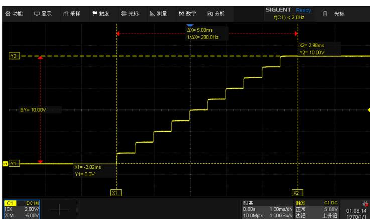
5. Refer to “Measurement Result”, in the **Result** > **Measure** interface, you can see the measurement results of 10 points as follows:
