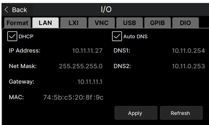
4. Set up DHCP, IP address, subnet mask, and gateway;
