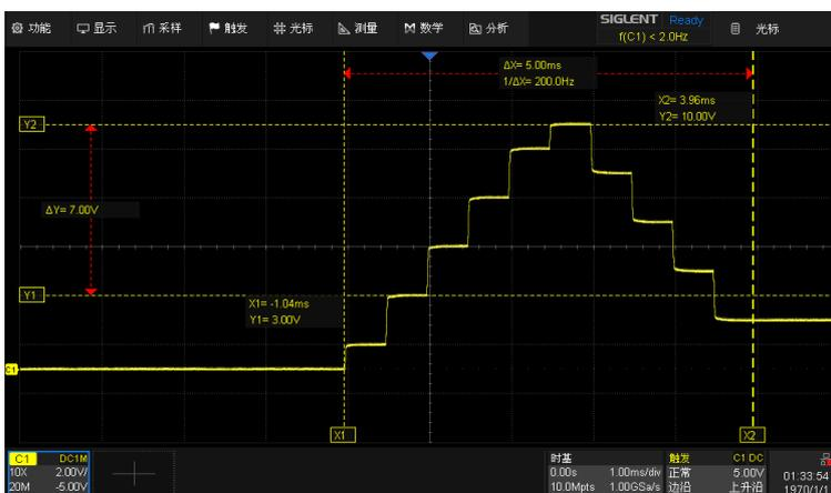
4. Refer to “Measurement Result”, in the **Result** > **Measure** interface, you can see the measurement results of 10 points as follows:
