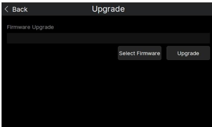
**Note:** Any operation that interrupts the upgrade process may cause the upgrade to fail or even prevent the machine from restarting, so please keep the USB flash drive in a stable state and the machine's power supply during the upgrade process.
