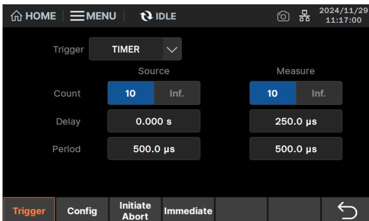
3. Refer to “[Trigger System Control](#)” to initiate the trigger system. Click **Initiate ALL** to start sweep output and measurement as follows:
