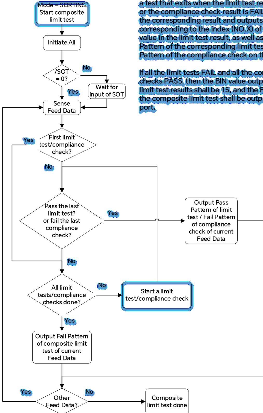
The composite limit test in the SORTING mode is a test that exits when the limit test result is PASS or the compliance check result is FAIL. It outputs the corresponding result and outputs the X value corresponding to the index (NO.X) of the BIN value in the limit test result, as well as the Pass Pattern of the corresponding limit test or the Fail Pattern of the compliance check on the DIO port.
