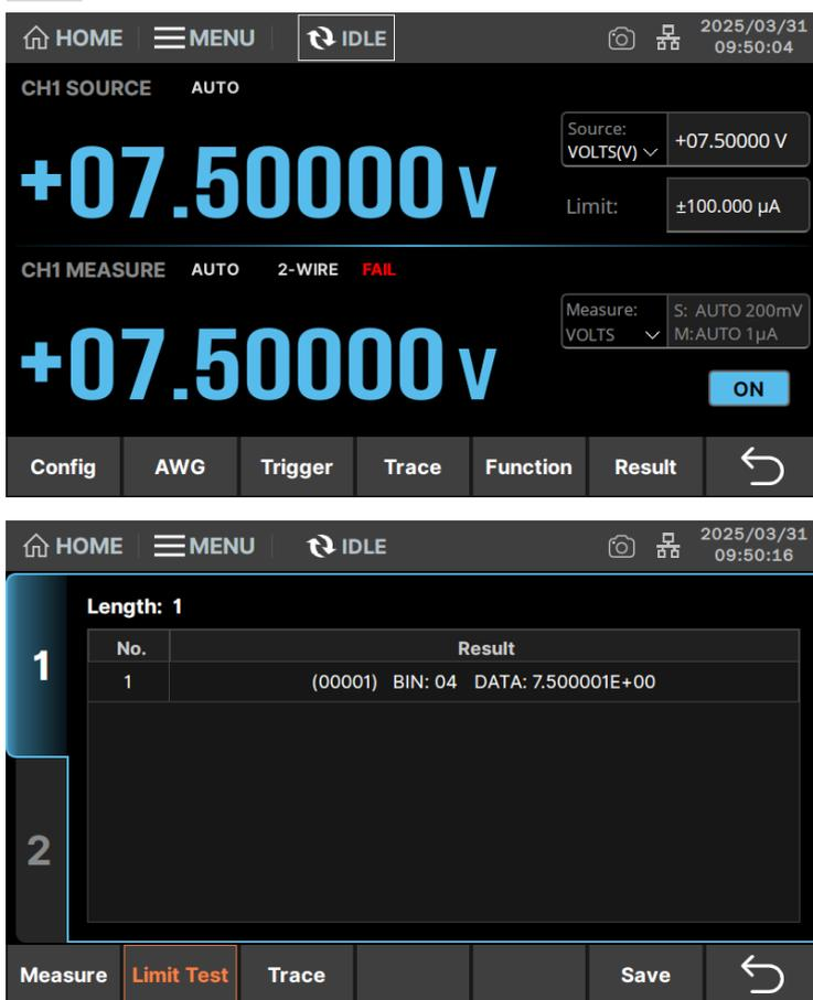
As shown, (00001) indicates the first data, and BIN: 04 indicates that the composite limit test ends in the 4th limit test because the test data “DATA” is not in the 4th limit test set for the range [4,7].
