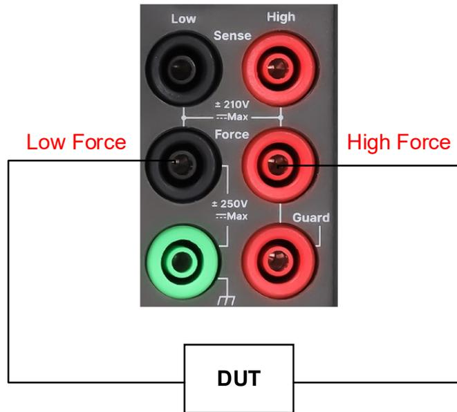
Figure 9-1 2-Wire Connection Diagram
