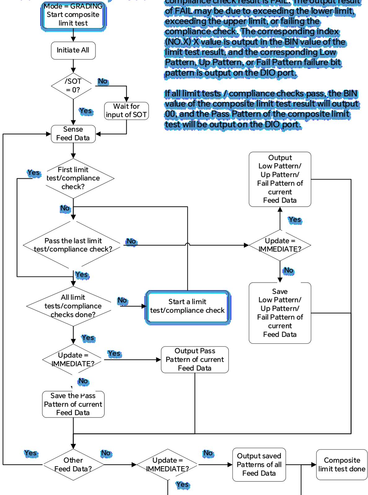
The composite limit test under the GRADING mode is a test that exits when a limit test/compliance check result is FAIL. The output result of FAIL may be due to exceeding the lower limit, exceeding the upper limit, or failing the compliance check. The corresponding index (NO.X) X value is output in the BIN value of the limit test result, and the corresponding Low Pattern, Up Pattern, or Fail Pattern failure bit pattern is output on the DIO port.
