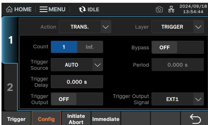
2. Select the channel to be set (1 or 2) to enter the single channel setting interface;
