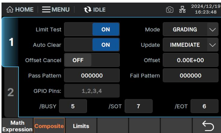
2. Refer to “[Limit Tests](#)”, in the **Function** > **Limits** interface, set each limit test/compliance test of NO.1-12, and this example sets NO.1-5, which is expressed as five tests for each measurement data respectively in one round of composite limit test, and the upper and lower limits of the test ranges are [1,10], [2,9], [3,8], [4,7], [5,6], which need to be set sequentially as follows:
