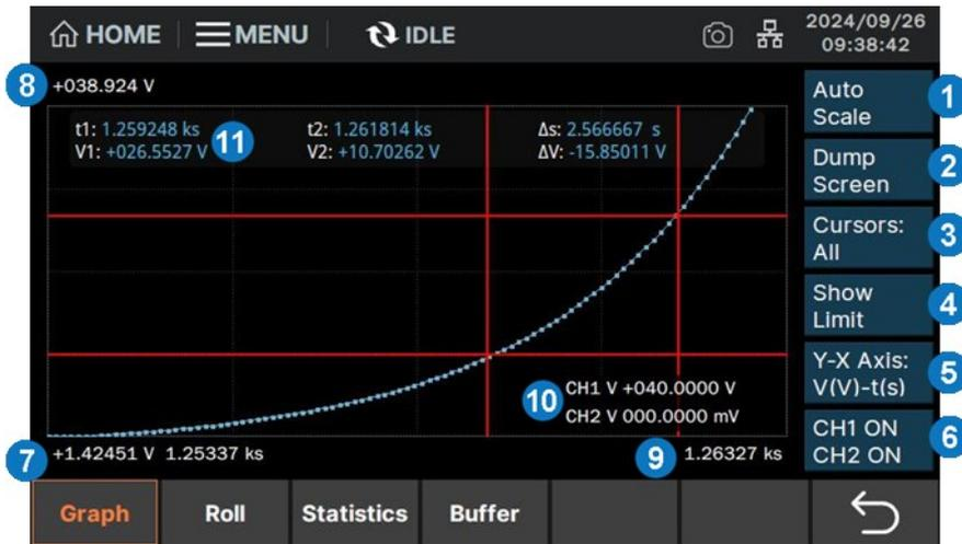
1. Auto Scale: Change the graphic scale to automatically fit the traces in the graphic.
