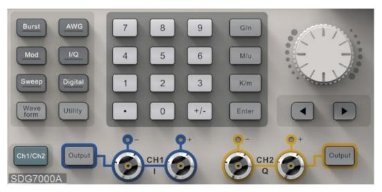
The SDG7000A Series Arbitrary Waveform Generator has integrated front panel buttons for frequently used functions, which can be used in conjunction with the touch screen for more efficient operation.
