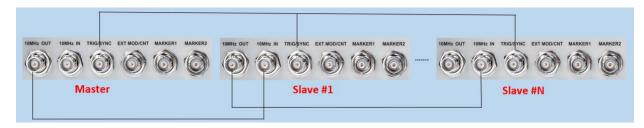
Figure 17-1 wiring diagram of multi-device synchronization
