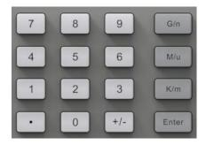
Use the numeric keypad to directly enter the value and order of magnitude of the selected parameter.
